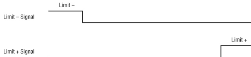
Figure 22: Limit - and Limit + TTL input signals.
