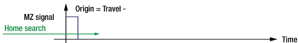
Figure 6: Minus end of run home search process.
