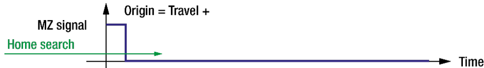
Figure 7: Plus end of run home search process.
