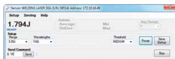
PC application energy screen
