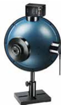
FPD detector mounted on IS6
